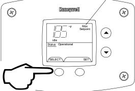
2a. Water Temperature Average (Displays average if there are two sensors - sensor temperature displayed if single sensor is used).
